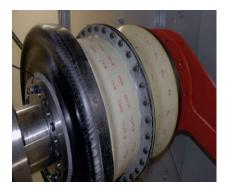
Figure 7 – A Composite Coupling on the Geislinger test bed.
