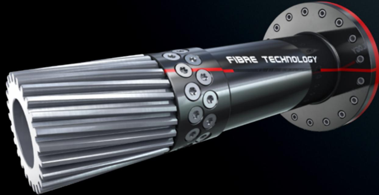
The Geislinger GESILCO® Silentshaft Coupling is our smartest solution for mitigating noise, vibration, and harshness for on-shore wind turbines. It effectively mitigates the sun shaft mode by lowering the torsional stiffness of the sun shaft, while it is no 'add-on' solution, and it is fully integrated to the gearbox.
