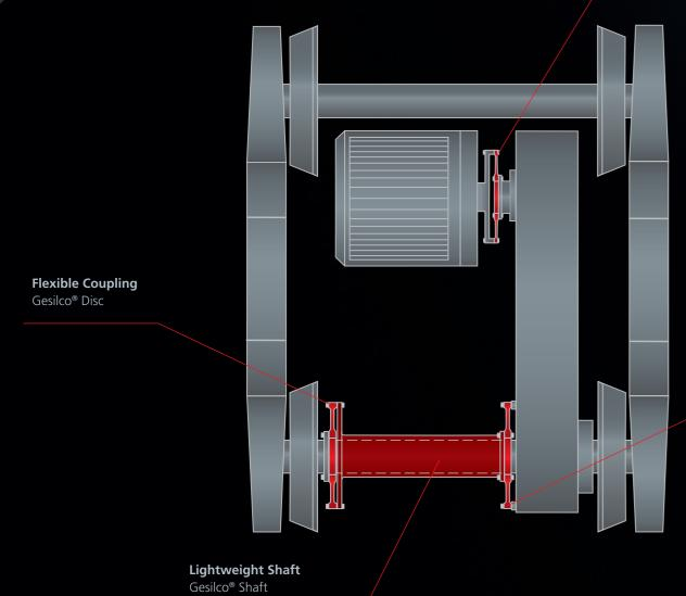
Flexible Coupling with electrical insulation Gesilco® Disc
