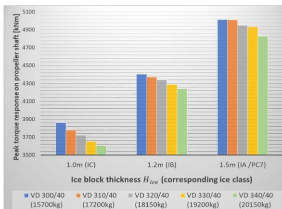
Figure 5. Comparison of peak torque responses on the propeller shaft for different viscous dampers
