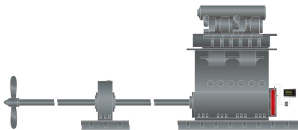
Figure 1. Principle layout of a two-stroke ship propulsion
