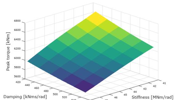
Figure 6. Peak torque response at propeller shaft
