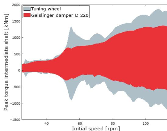
Figure 4. Worst case detection: Peak torque response at the intermediate shaft
