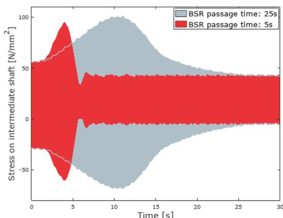
Figure 3. Stress response on the intermediate shaft over time for two different BSR passage times.
