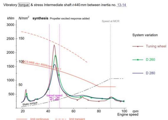
Figure 2. Steady-state TV analysis: Comparison of vibratory torque and stress responses for systems with tuning wheel and 2 different spring dampers
