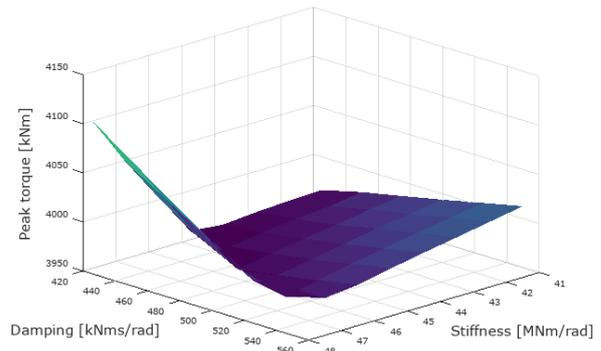
Figure 7. Peak torque response at cylinder 1
