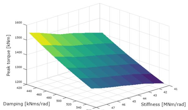
Figure 8. Peak torque response at damper D 340
