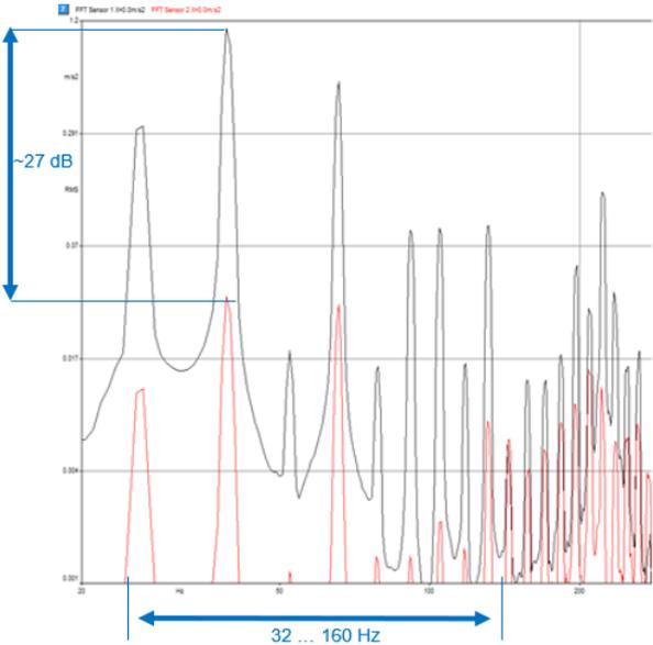
Figure 4 – The acceleration caused by engine noise measured in the front (black) and in the rear (red) of a coupling on the Geislinger test bed.
