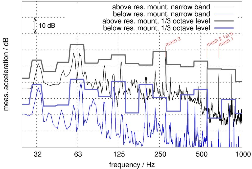
Figure 9 – Measured structure borne noise levels for the AED (1).
