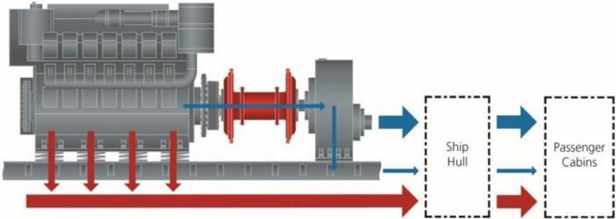
Figure 2 – The path of structure borne noise on a ship. Red: primary path, blue: secondary path.
