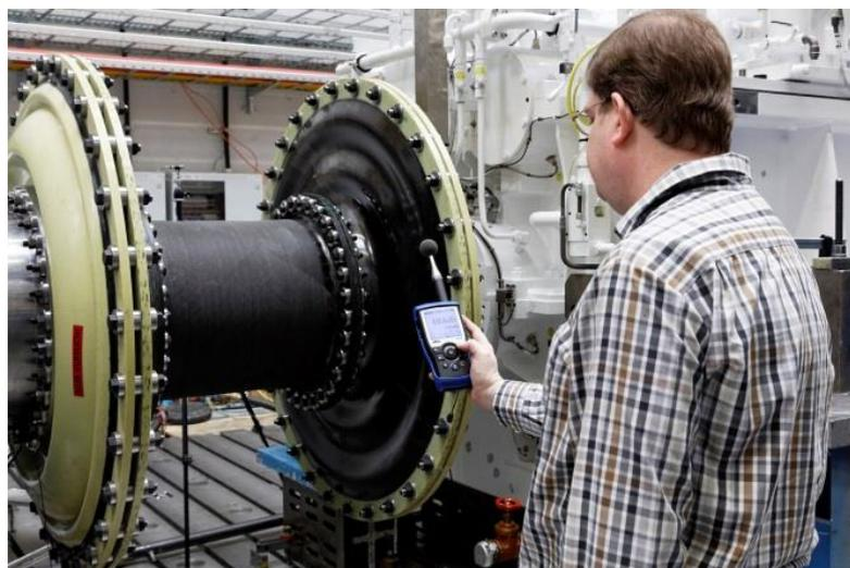
Figure 8 – A Silenco® coupling tested with the Renk AED.
