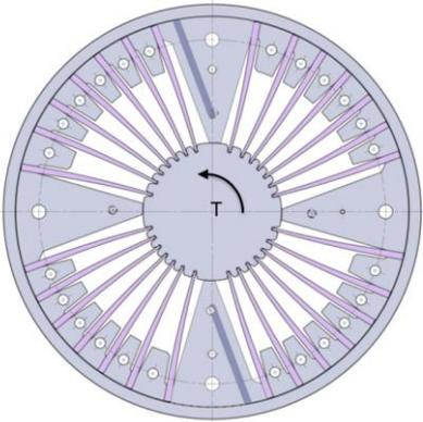
Figure 5 – The Geislinger NCA coupling.
