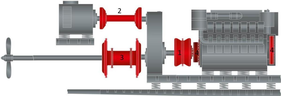
Figure 3 – An example of a powertrain in a mega yacht with different couplings (2). The lightweight composite misalignment coupling no. 1 in figure 3 reduces the engine noise.
