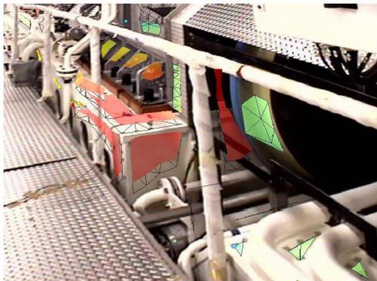
Figure 10 – Validation of the transmission loss of a Geislinger coupling during a sea trial (1)
