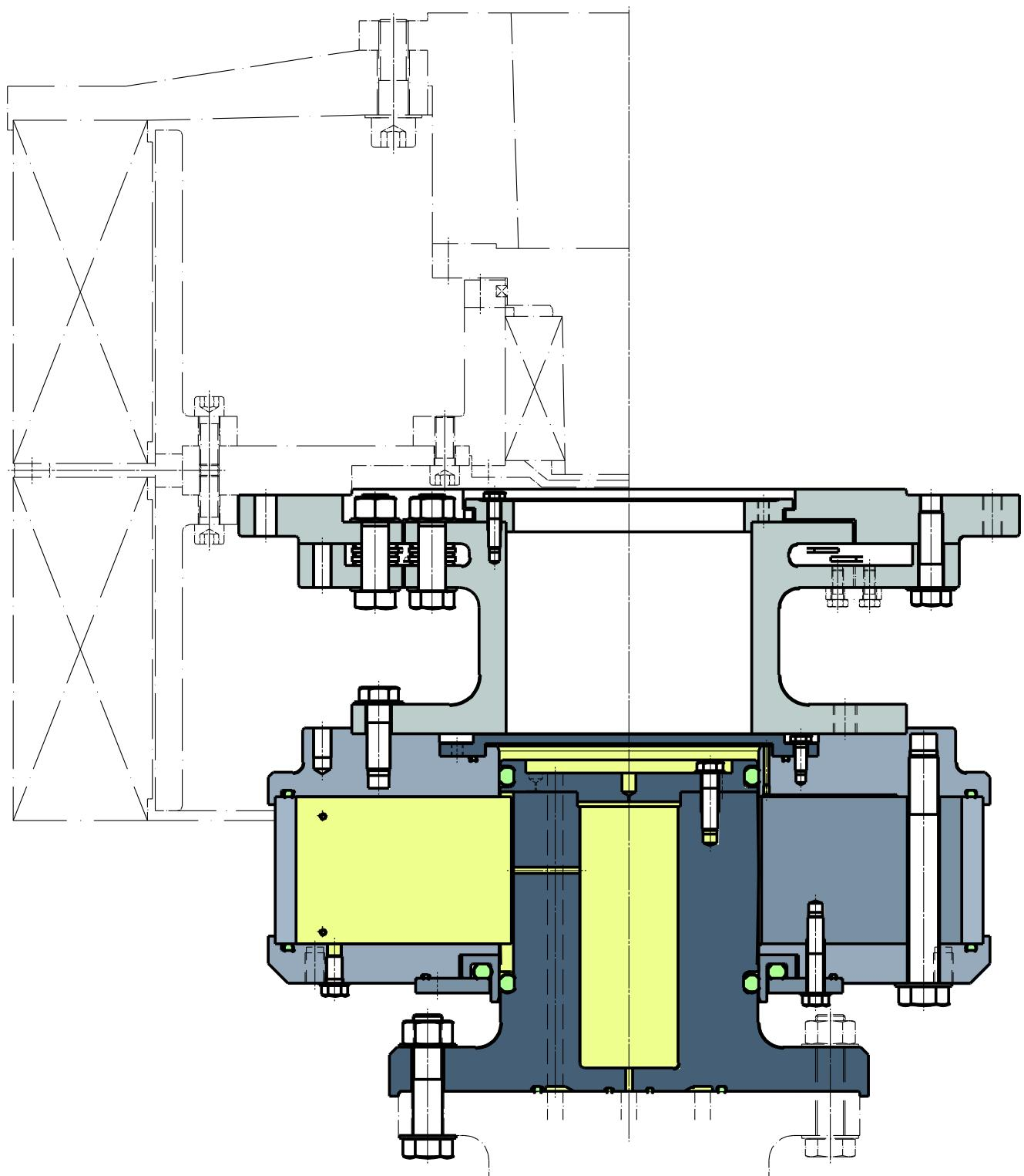
■ Geislinger Flexlinks with Gesilco composite shaft
