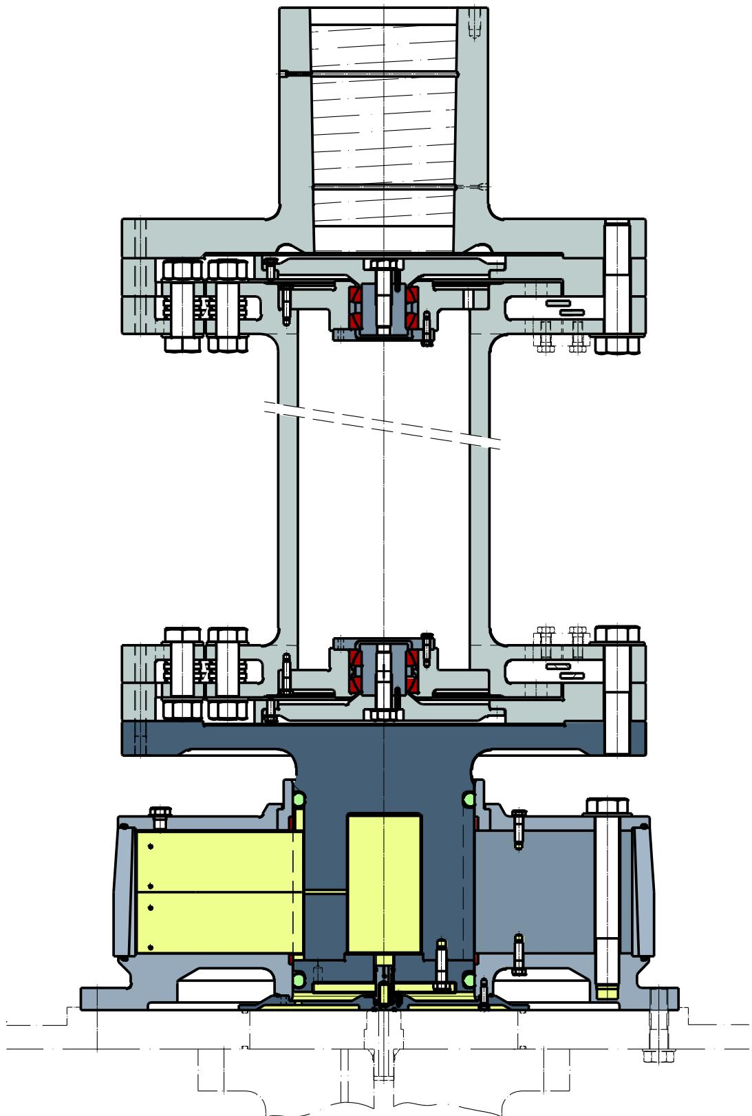
■ Geislinger BC Coupling + Geislinger Flexlink K6 with long shaft
